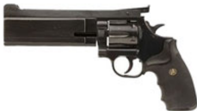
Examples of customised revolvers - slab sided and bull barrels, customs sights and lots of internal trigger work
