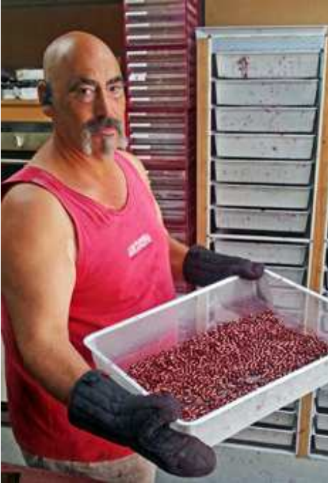
John bakes the red lubricant coating onto the projectiles in ovens in his - they are still hot so heavy gloves are essential.
